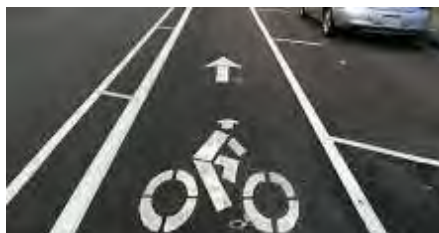
Example of Buffered Bike Lanes – Source: Kimley-Horn
