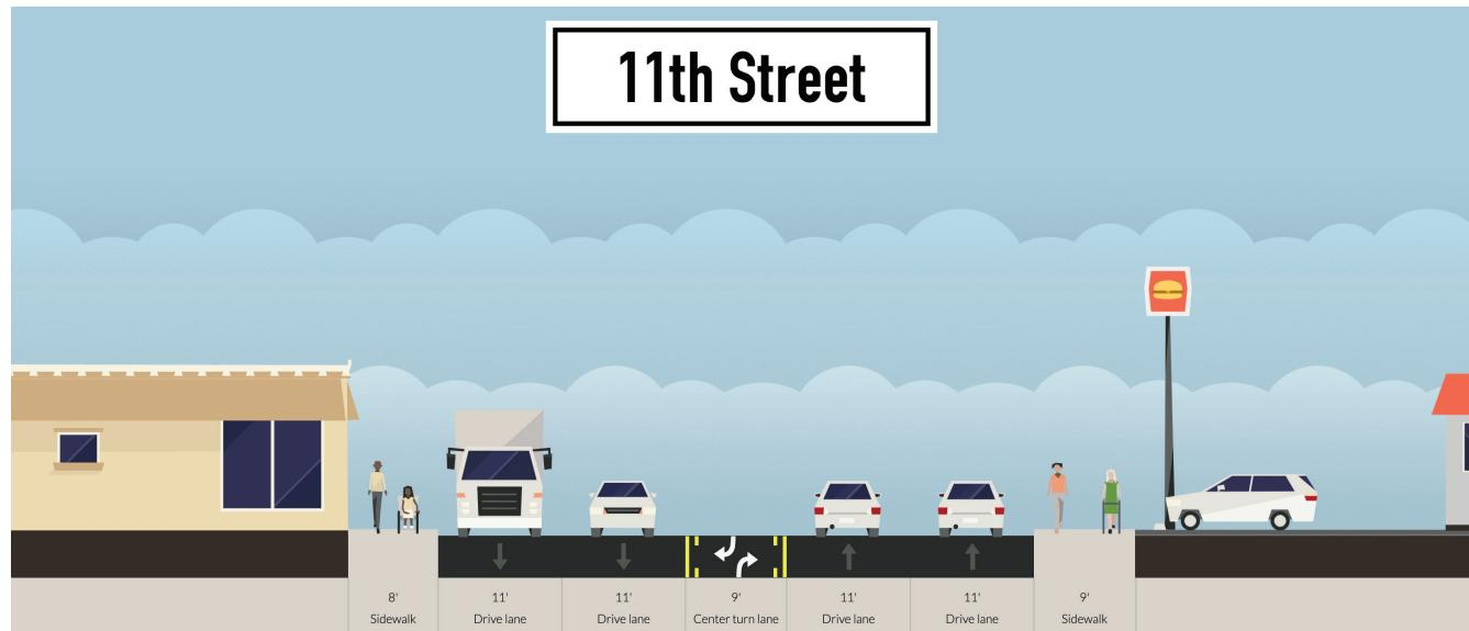
Figure 3-3: 11th Street Section Showing Mid-Block Improvements
